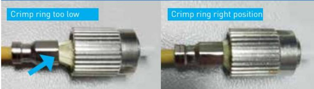
Figure 5: Non-compliant to standard dimension could cause
