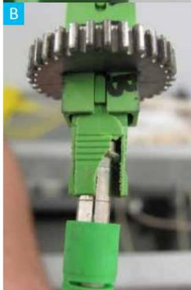
Figure 8: Improper crimp ring placement during crimping
